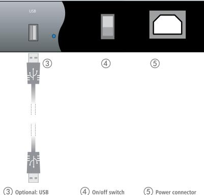
(3) Optional: USB You can use the USB interface to connect a compatible USB cellular modem, a USB printer your PC or a LAN switch. or a USB flash drive for device configuration.
